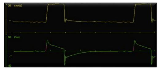
Figure 2. The start of each insufflation is NOT preceded by any notch on the pressure-time curve.
